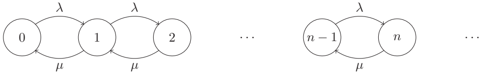
Figure 2.1.3. Flow diagram for the M/M/1 queue.
