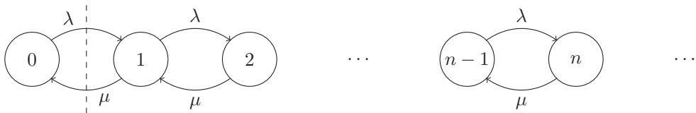
Figure 2.1.4. Flow diagram of the probability flux for the M/M/1 queue.
