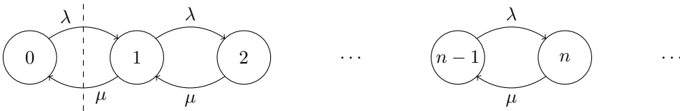
Figure 3.2.4. Flow diagram of the probability flux for the M/M/1 queue.
