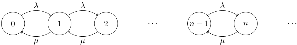
Figure 3.2.3. Flow diagram for the M/M/1 queue.
